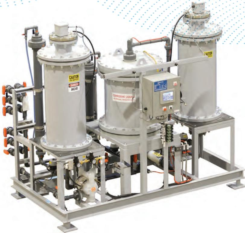
The AnoPur™ unit is a small, skid-mounted device that connects directly to an anodizing tank to continuously remove aluminum as it is dissolved in sulfuric acid. The system relies on Eco-Tec ion exchange resin technology to effectively remove metal contaminants and purify and recycle sulfuric acid.
